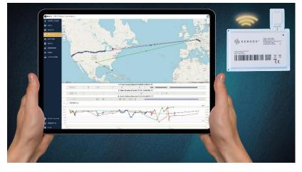
SENSOS, which has developed an intelligent, digitally networked shipping label in the size of a credit card. The smart shipping label, which is only a few millimeters thick, can be easily and securely affixed to a wide variety of consignments. Thanks to its integration into the BOX ID Cloud software, precise localization, exact condition monitoring – for example with regard to temperature or impact and the integrity of the packaging – can be carried out to the second.
